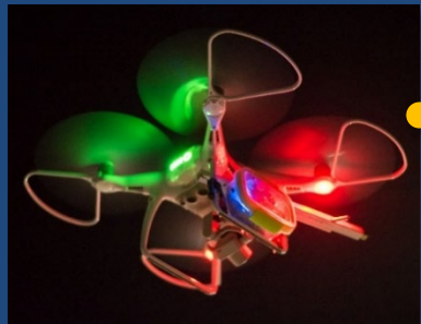
Quadcopter-based vertical temperature sounding over the city
